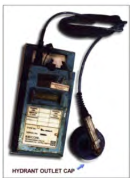
Typical pressure logger installation with hydrant cap and flexible hose
