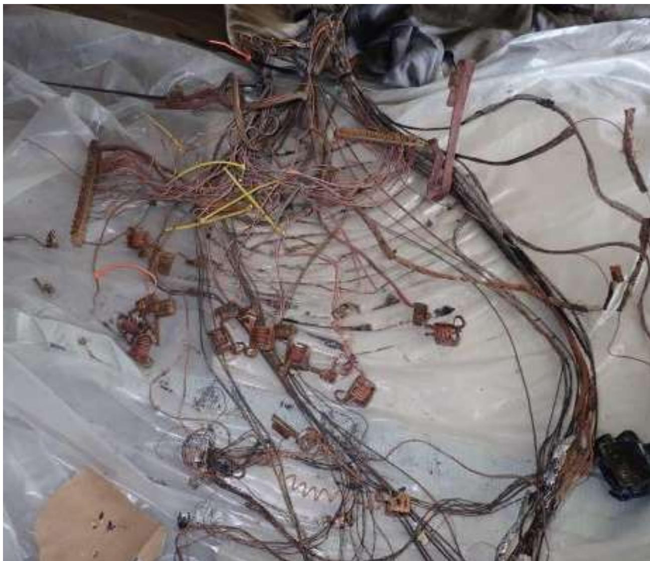
Image showing the remains of the top half of the consumer unit
