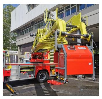
The 64m TL cage must not be removed as Rescue loader and Safety 5 is not compatible with this appliance.
