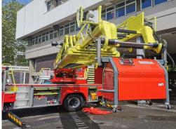
5.30 The 32m TL has a lifting eye at the head of the top extension which has a safe working load of 500kg.
