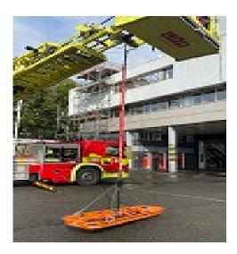
5.29 Additionally, the 32m TL will carry the 'safety 5' piece of equipment. This enables safe working at height when other line operations options are not available. TL operators are not trained in level two-line operation. TL Magirus Safety Five Safety System.
